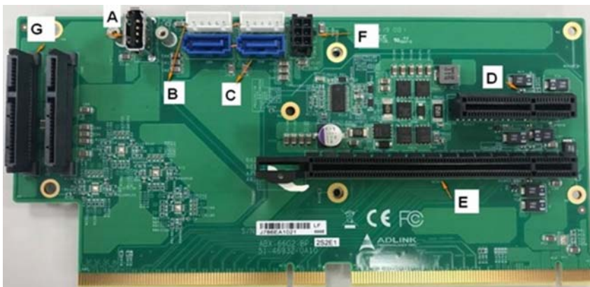
Figure 3-11: 2-slot Backplane Board Connectors
