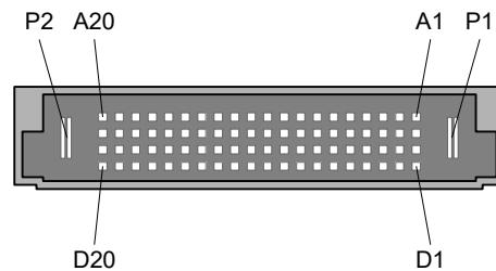
**Figure 11:** Internal Power Backplane Connector
