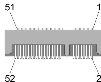
**Figure 13:** mSATA Full-Mini Card Socket Connector (JAE, MM60-52B1-E1-R650)
