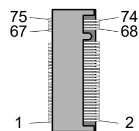
**Figure 12:** M.2 Key M Socket Connector (TE, TE12199230-6)
