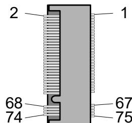
**Figure 14:** MPL AGs TPM Module Socket Connector (TE, TE12199230-6)
