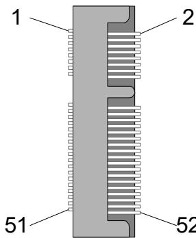
Figure 21: mPCIe Full-Mini Card Socket Connector (JAE, MM60-52B1-E1-R650)
