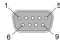
**Figure 5:** Serial Port Connector (DSUB 9 Male)
