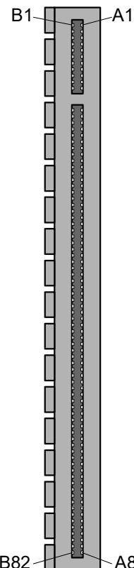
Figure 19: PCIe PEG Port Connector (Samtec, PCIE-164-02-F-D-EMS2-BG)
