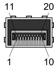
**Figure 10:** SFP+ Cage Connector ((Samtec, MECT-110-01-M-D-RA1 and SFPC-SL)
