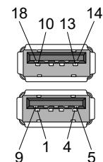
**Figure 6:** Dual USB 3.0 (Type A) Connector (TE, 1932355-1)
