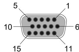
Figure 7: VGA Connector (Compona, 363062)
