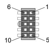
**Figure 16:** Power Connector for SATA Devices (Samtec, IPL1-105-02-S-D)
